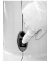
Intensive sterilisation is in step 4 (dwell time): Simultaneously press and hold the intensive sterilisation key and hydrocolloid key.
